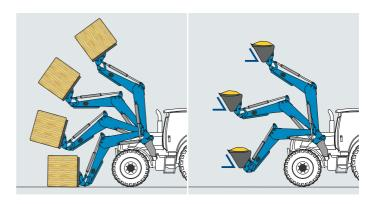
NSL (NON SELF LEVELLING SYSTEM) Robust and simple to operate.
